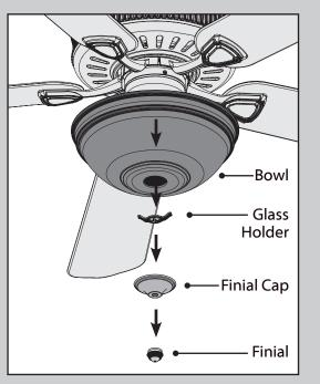
**Changing the bulbs** - unscrew the finial and remove it from the threaded rod. Remove the finial cap and unscrew the glass holder while supporting the globe with your other hand. Carefully remove the globe. Unscrew bulbs and replace with bulbs of the same type and wattage. Reinstall the globe assembly.
